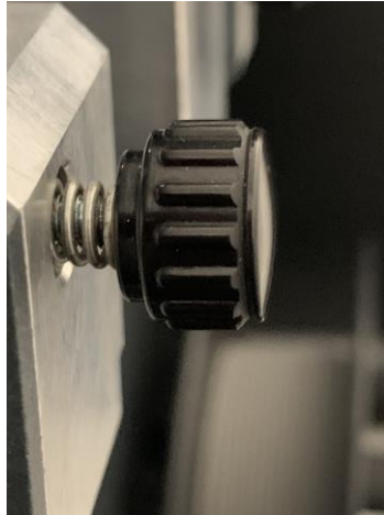
Fig. 2: Screw on dual gear drive loosened to reduce pressure and grinding on filament while still driving the filament for effective feeding through the printing nozzle
