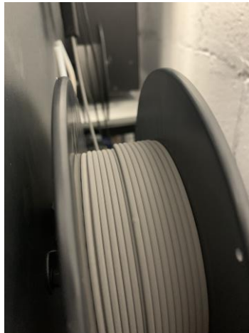
Fig. 1: CMG Tech-X HMs metal filament spool on holder behind BCN3D Epsilon 3D printer
