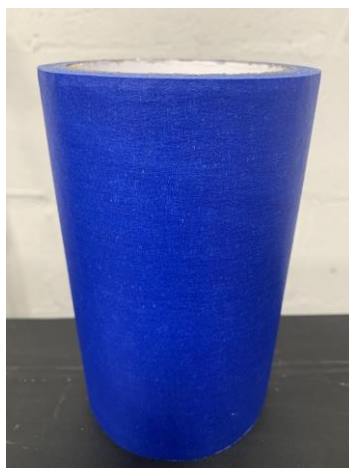
Fig. 3: Blue painter's tape for use as bed adhesion material when printing CMG Tech-X HMs metal filament on BCN3D Epsilon 3D printers. The bed temperature should be set to 20 °C.
