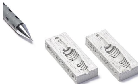
Fig. 1: Sintered mould cavity printed with CMG Tech-X H13 HMs filament.
